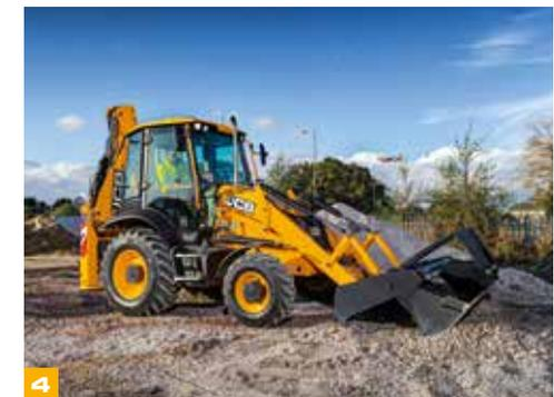
Tractive effort in the pile is maximised with the variable flow hydraulics and JCB's Stage V Dieselmax engine.
